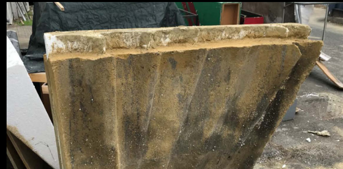
Robotically fabricated mould for concrete casting by Abdullah bin Musa.
